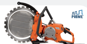
PETROL-POWERED HUSQVARNA K 7000 RING 230/400V, 5.5 kW (3-phase)/3 kW (1-phase), 13.1/12.4 kg, blade size 350/425 mm, cutting depth 270/325 mm.
