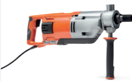
ELECTRIC-POWERED HUSQVARNA DM 220 1850 W, 1-phase, recommended drill diameter 150 mm, handheld 80 mm, 7.5 kg.
