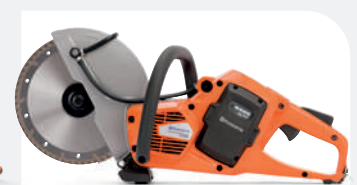
POWER CUTTER HUSQVARNA K 535i 3.5 kg, blade size 230 mm, cutting depth 76 mm.
