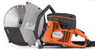
PETROL-POWERED HUSQVARNA K 770 DRY CUT 74 cc, 3.7 kW, 12.0 kg, blade size 305 mm, cutting depth 123 mm.
