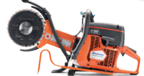
PETROL-POWERED HUSQVARNA K 760 CUT-N-BREAK 74 cc, 3.7 kW, 11.1 kg, blade size 230 mm, cutting depth 270 mm.
