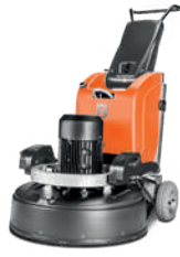
ELECTRIC-POWERED HUSQVARNA HTC 950 RX 15kW, 380-415, 440-480V, 3-phase, grinding width 920mm, grinding disc 4 x 270mm, 600kg.
