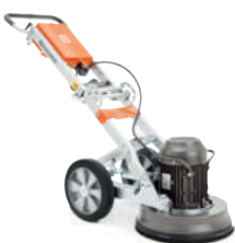
ELECTRIC-POWERED HUSQVARNA PG 400 4kW, 400V, 3-phase, grinding width 400mm, 115kg.
