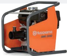
PETROL-POWERED HUSQVARNA AMG 3200 Drive unit for AA and AZ vibrators. 2.8kW, 15 kg.
