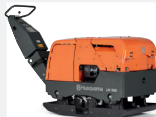
DIESEL-POWERED HUSQVARNA LH 700 11kW, 780kg.
