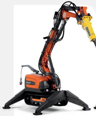
HYDRAULIC-POWERED HUSQVARNA DXR 315 27 kW, 2020 kg, reach 5.5/5.2 m up/forward incl. tool.
