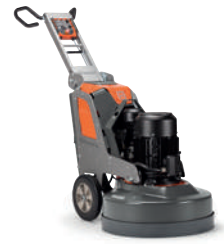
ELECTRIC-POWERED HUSQVARNA PG 830 16.5kW, 380-415V, 3-phase, grinding width 800mm, grinding disc 3 x 270mm, 556kg.
