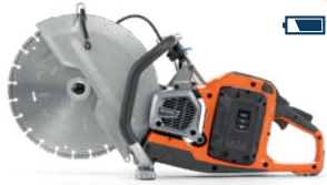
BATTERY-POWERED HUSQVARNA K 1 PACE 7.2/7.4 kg, blade size 300/350 mm, cutting depth 121/145 mm. PACE 94V battery system.
