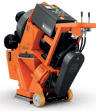
HYDRAULIC-POWERED HUSQVARNA BLASTRAC EBE 350S 11kW, 400V, 32A, working speed 1–30 m/min, working width 350mm, 415kg.
