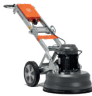
ELECTRIC-POWERED HUSQVARNA PG 510 4.0/2.2kW, 400/220V, 3-phase/1-phase, grinding width 515mm, grinding disc 3 x 230mm, 133/120kg.
