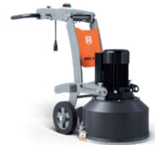
ELECTRIC-POWERED HUSQVARNA BMG 444SC 2.2kW, 230V 16A, grinding width 444mm, 132/135kg. Fixed speed/speed control.
