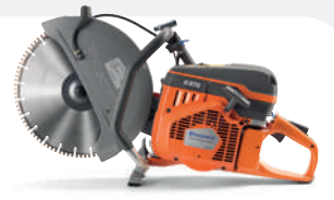
PETROL-POWERED HUSQVARNA K 970 94 cc, 4.8 kW, 11/11.6 kg, blade size 350/400 mm, cutting depth 125/155 mm.
