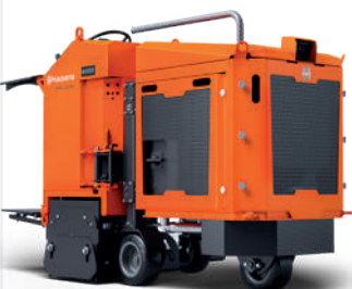
ELECTRIC-POWERED HUSQVARNA BMP 4000RC Remote controlled, 30kW, 400V/63A, 380mm working width, 1550kg.
