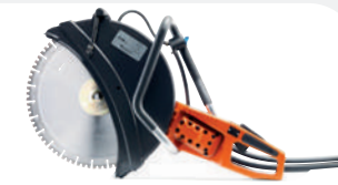
HYDRAULIC-POWERED HUSQVARNA K 2500 150 bar/40 l/min, 5.2 kW, 8.3 kg, blade size 400 mm, cutting depth 145 mm.
