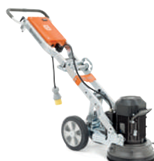
ELECTRIC-POWERED HUSQVARNA PG 280 3/2.2kW, 400/220V, 3-phase/1- phase, grinding width 280mm, 70kg.
