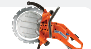
HYDRAULIC-POWERED HUSQVARNA K 3600 MK II 150 bar/40 l/min, 4.3 kW, 8.3 kg, blade size 370 mm, cutting depth 270 mm.
