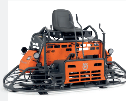
PETROL-POWERED HUSQVARNA CRT 48 Ideal for finishing surfaces 1000–1900 m 2 . Featuring a superior mechanical steering system and balanced power-to-weight ratio. 27.6kW, 2×1220mm, 579kg.
