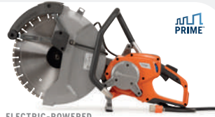
ELECTRIC-POWERED HUSQVARNA K 7000 SMARTGUARD 230/400V, 5.8 kW (3-phase)/3 kW (1-phase), 5.1 kg, blade size 400 mm, cutting depth 145 mm.
