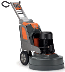
ELECTRIC-POWERED HUSQVARNA PG 830 S 11kW, 380-415V, 3-phase, grinding width 800mm, grinding disc 3 x 270mm, 497kg.
