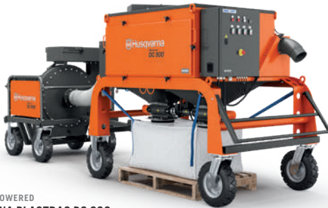
ELECTRIC-POWERED HUSQVARNA BLASTRAC DC 900 17kW, 400V, 32A, 860kg.
