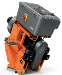
ELECTRIC-POWERED HUSQVARNA BLASTRAC EBE 350EX 11kW, 400V, 32A, working speed 1–15 m/min, working width 350mm, 450kg.
