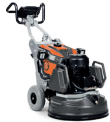
ELECTRIC-POWERED HUSQVARNA HTC 5 4.0/2.2kW, 400/220V, 3-phase/1-phase, grinding width 515mm, grinding disc 3 x 230mm, 122/179kg.
