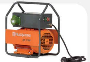
ELECTRIC-POWERED HUSQVARNA CF 11 Output 42 V–3–200 Hz, 0.8 kVA, 11A, 18kg, 1 outlet.
