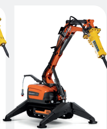
HYDRAULIC-POWERED HUSQVARNA DXR 305 27 kW, 1960 kg, reach 5.2/4.9 m up/forward incl. tool.
