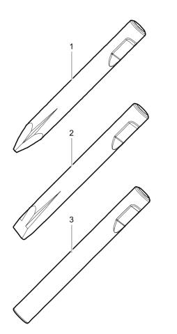
Ø=145 mm, L= 665 mm, LT=1230 mm, Wt=139.0 kg Ø=5.71 inch, L=26 inch, LT=48.43 inch, Wt=306.4 lb
