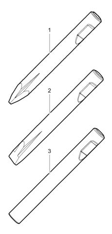
Ø=155 mm, L=640 mm, Lt=1350 mm, Wt=168.0 kg Ø=6.10 inch, L=25 inch, LT=53.15 inch, Wt=370.4 lb
