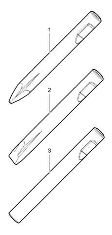
Ø=170 mm, L= 720 mm, LT=1500 mm, Wt=231.5 kg Ø=6.69 inch, L=28 inch, LT=59.06 inch, Wt=510.4 lb
