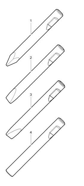
Ø=190 mm, L=730 mm, LT=1580 mm, Wt=306.0 kg Ø=7.48 inch, L=29 inch, LT=62.20 inch, Wt=674.6 lb
