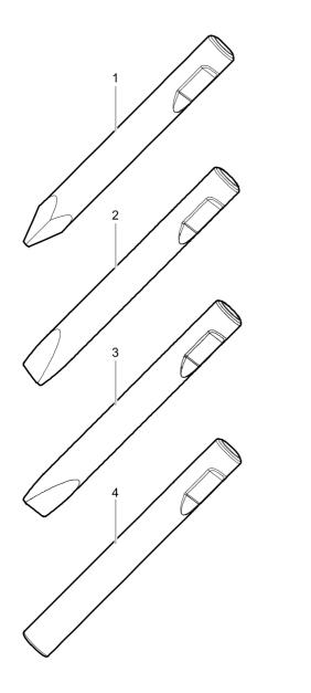
Ø=190 mm, L=790 mm, LT=1580 mm, Wt=306.0 kg Ø=7.48 inch, L=31 inch, LT=62.20 inch, Wt=674.6 lb
