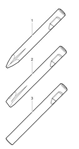
$\varnothing$ =210 mm, L=935 mm, LT=1800 mm, Wt=417.0 kg  $\varnothing$ =8.27 inch, L=37 inch, LT=70.87 inch, Wt=919.3 lb
