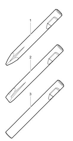
Ø=110 mm, L= 630 mm, LT=1100 mm, Wt=73.0 kg Ø=4.33 inch, L=25 inch, LT=43.31 inch, Wt=160.9 lb
