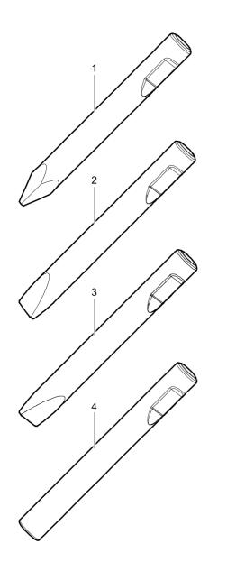
Ø=110 mm, L= 570 mm, LT=1040 mm, Wt=69.0 kg Ø=4.33 inch, L=22 inch, LT=40.94 inch, Wt=152.1lb
