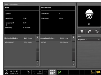
User: sets the control system language. Logs in users to the control system and shows user information.
