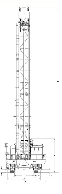
'Approximate shipping dimensions for crated PV-311 (actual dimensions will vary based on rig configuration).
