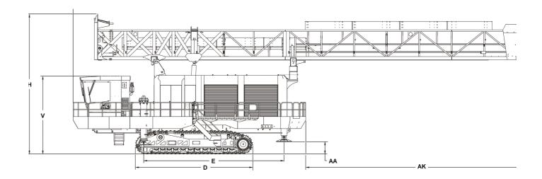
Approximate shipping dimensions for crated PV-316 with 75 ft tower (actual dimensions will vary based on rig configuration).
