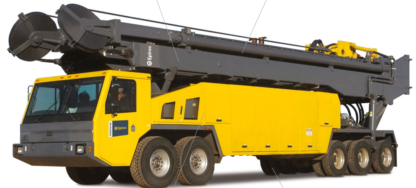
Tri-axle drive on the carrier rear axle sets ensures positive traction for maneuvering in difficult oilfield terrain.
