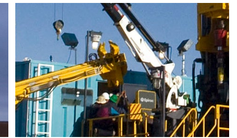
The pipe skate features rapid deployment and hands-free pipe handling from the pipe racks all the way to the pipe connection. Skate operations can be controlled from the ground or the rig work floor via a wireless remote controller.
