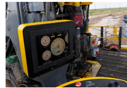
A robust, military-grade control console monitor displays drilling parameter gauges, engine parameters and drilling system diagnostics.
