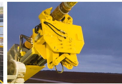
The Driller has complete control over the connection process by clamping and extending the drill pipe to the top drive and threading it into the pipe for a secure connection before bringing the drill pipe in through the drill floor.
