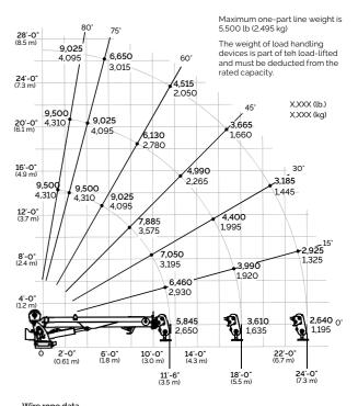
**Wire rope data** Diameter: 0.44 in (11.2 mm), non-rotation resistant Minimum breaking load: 20,400 lb (9,253.3 kg)
