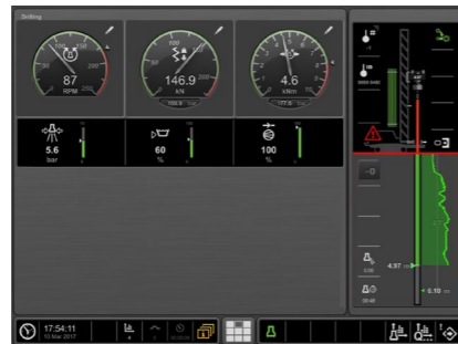
Drilling: shows information about pressures and flows for various systems during drilling.
