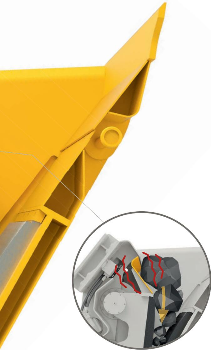
To increase throughput, a **moving sliding plate** continuously guides material to the crushing jaw.
