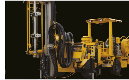
Versatile positioning system supplies 3 meters parallel in horizontal and 360° ring pattern.
