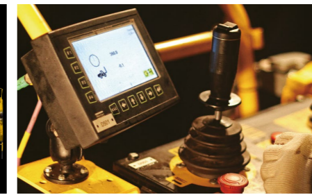
Digitized angle reading system helps operators to fulfill more accurate hole angle and depth.
