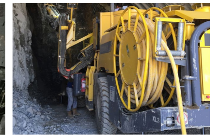
Maintenance-friendly design makes the service work safe and easy. All service points are reachable from ground level
