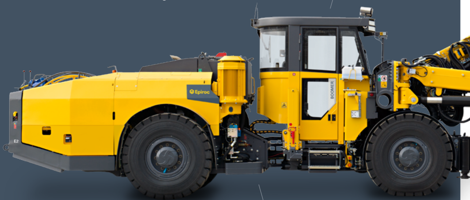
Articulated steering for greater agility in tighter tunnel dimensions
