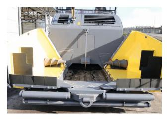
Two augers for homogeneous material flow.
