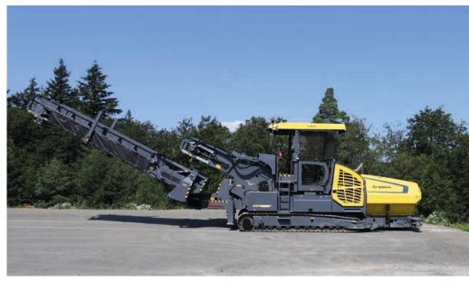
BMF 2500 S offset with slewing conveyor belt for the short version.
