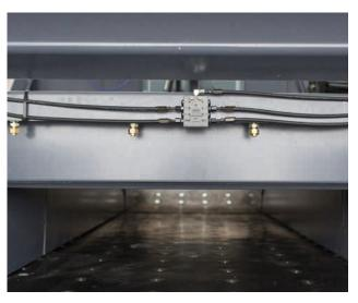
Cleaning at the push of a button: the belt cleaning system.
