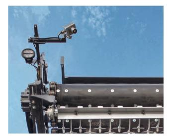
Automated material flow: the filling level sensor.
