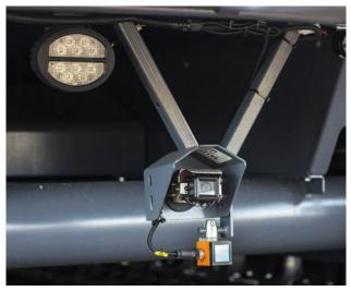
Synchronised speed: the distance sensor.
