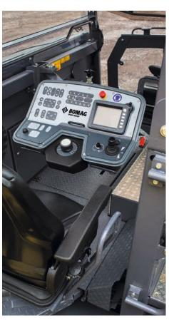
Comfortable: rotating seat with control panel.
