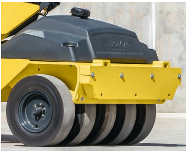
To increase stability, the ballast compartments have been positioned extremely low, as shown here above the front axle.
