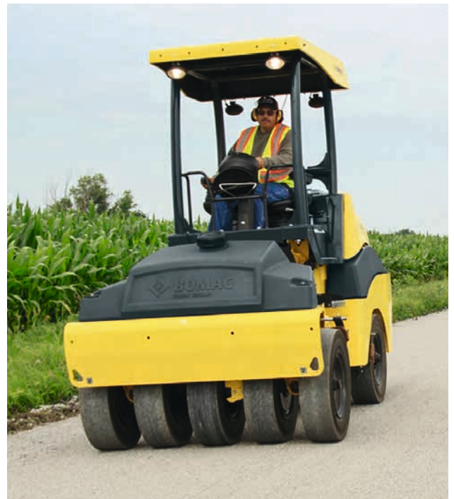
The BW 11 RH-5 provides perfect compaction and a smooth and even surface finish.
