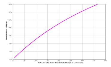
Peak motor starting (kVA) based on x% voltage dip power factor at 0.3
